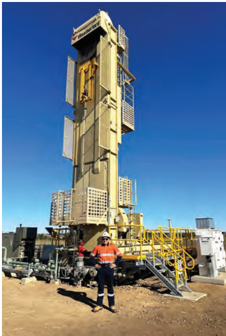
Fig. 1. The Weatherford Rotaflex® long-stroke pumping unit delivers a stroke length from 180 in. to 366 in. (4.6 m to 9.3 m) for efficient pumping in deep, high-volume and problematic wells. Its long, slow pump stroke allows more time for fluids to enter the pump intake, which increases pump fillage and lifting efficiency.
