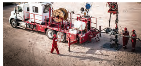
Fig. 2. Capillary tubing unit deployed for chemical injection—enabling precise, rigless well remediation as part of the MARS system's targeted intervention capabilities.
