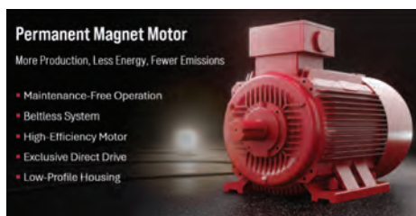
Fig. 2. Weatherford PMM-RF for Rotaflex® provides an AC synchronous, direct-drive motor that uses magnets embedded on the surface of the motor rotor to create a continuous magnetic field. The PMM-RF delivers up to 95.2% efficiency with a 0.95 power factor than can provide up to 30% less energy consumption, compared to conventional induction motor systems.
