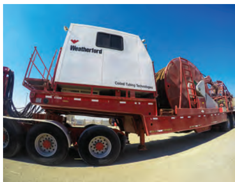
Fig. 2. Flexible conveyance capabilities, including coiled tubing and capillary units, eliminate the need for a rig.
