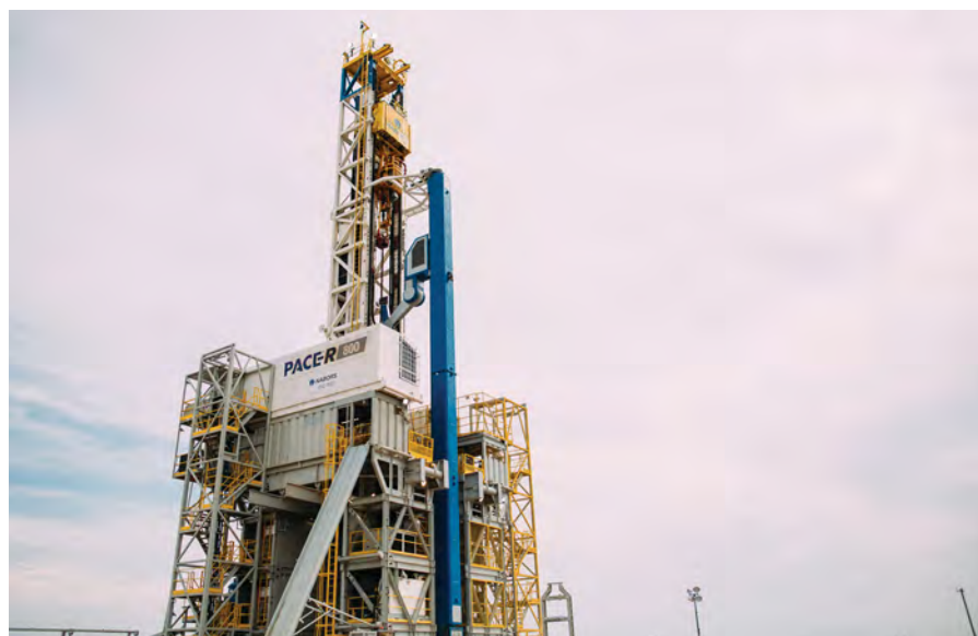
Fig. 1. The rebound in U.S. drilling is being supported by continued technical innovation, such as the Nabors PACE®-R801 (pictured here), the world's first fully automated land rig, which successfully drilled its first well on a test pad in Midland County, Texas, last October. Image: Nabors Industries.
