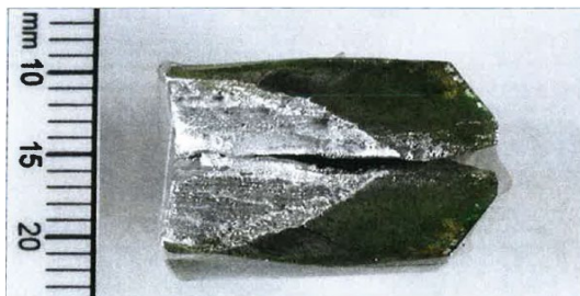
Fig. 7: Crack surfaces after opening the crack
